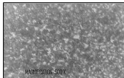
Figure 03 - Microstructure of conventionally treated EN 31 specimen at 100X and 500X magnification
