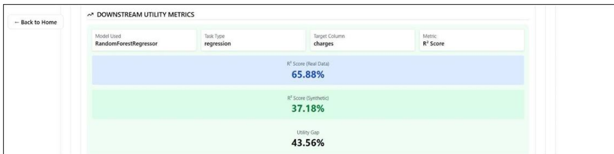
FIGURE 4: SecureSynth Downstream Utility Evaluation — RandomForestRegressor achieves R 2 Score of 65.88% on real data and 37.18% on synthetic data, with a utility gap of 43.56% on the insurance charges prediction task.
