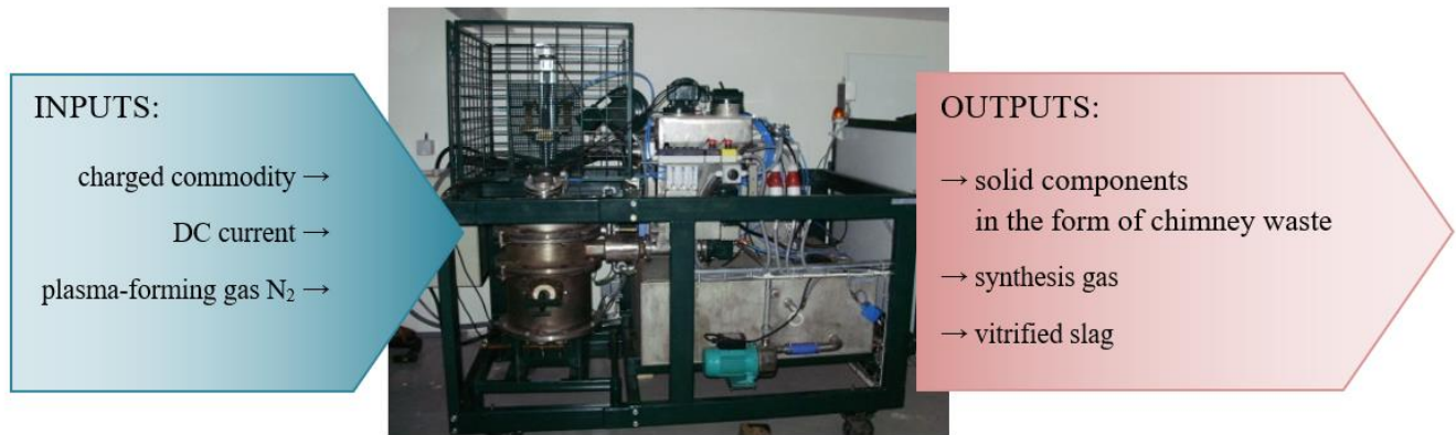
FIGURE 1: Laboratory plasma reactor with its inputs and outputs
