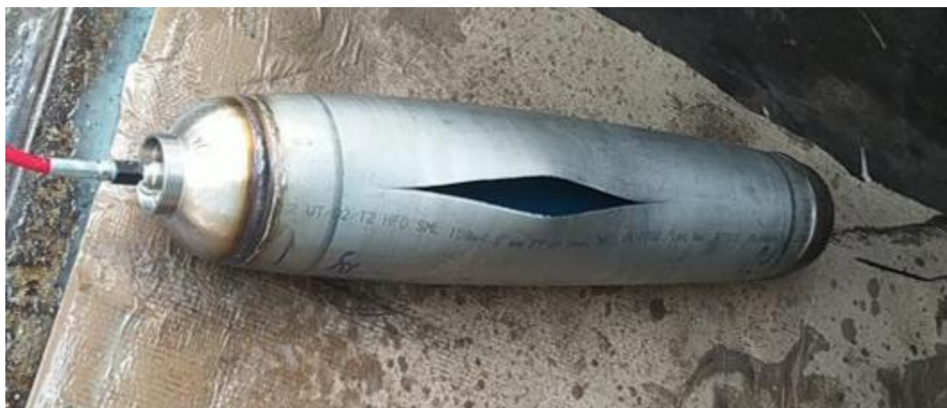
FIGURE 2: Result of hydraulic test until failure
