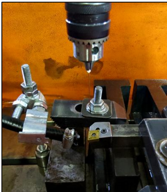
FIGURE 1: DRILLING OF INSERTS USING ELECTRICAL DISCHARGE MACHINING
