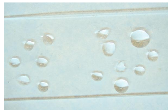
FIG. 8. WATER DROPLETS ON PMMA AFTER TREATMENT IN CHLOROFORM VAPOR. LEFT - UNTREATED AREA, RIGHT - PROCESSED
