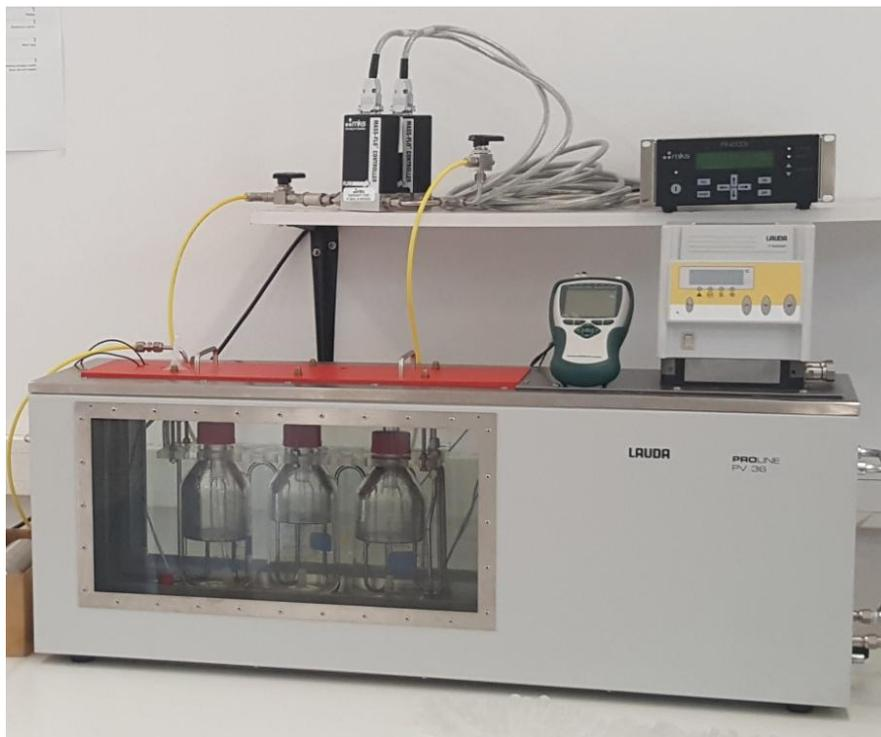
**FIGURE 1: System for monitoring the ethanol concentration.**
