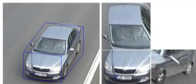
FIGURE 2: 3D bounding box constructed around vehicle, and then split so the three views form a three-view drawing.
