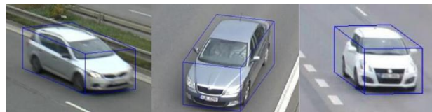
FIGURE 11: Examples of 3D bounding box construction
