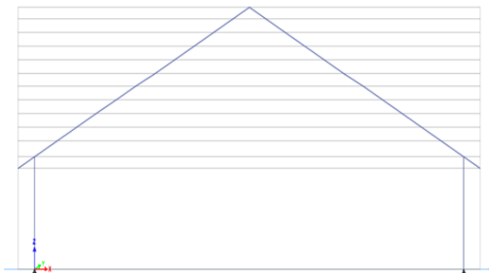
FIGURE 1: Frame with 22° slope
