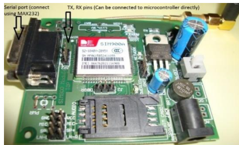
FIGURE 4: GSM Module SIM900
