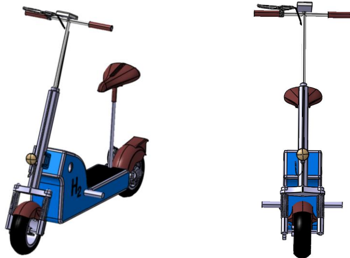
FIGURE 2: Concept of a hybrid two-wheeler powered by a fuel cell and an electric motor
