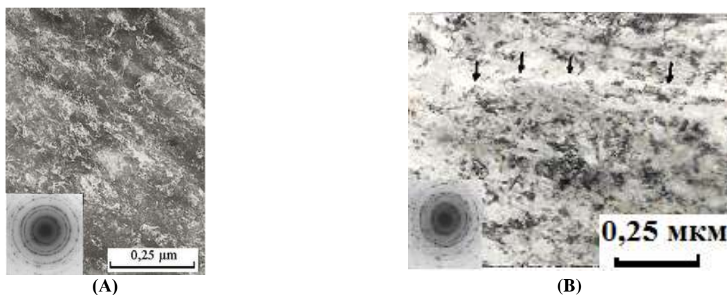
FIGURE 2: Formation of nanostructures at t = 0.9 ks on the nickel surface at nominal contact pressure: a) 84 kPa; b) 168 kPa
